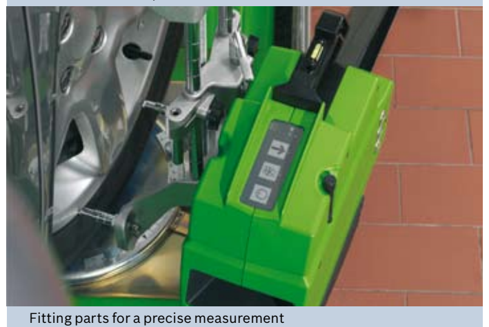
Sensor heads with protective rubber
