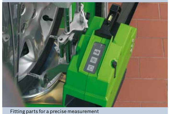
Sensor heads with protective rubber
